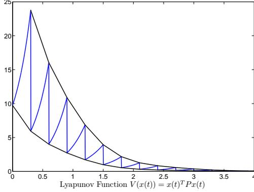
Fig. 1. Continuous-time Lyapunov function  $V$  (plain) for Example 3.7 and the discrete-time envelopes (dashed). The discrete-time envelopes are monotonically decreasing while the continuous-time function is highly non-monotonic along the flow of the system.
