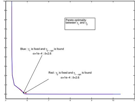
Fig. 8. Pareto optimality, xaxis= $\gamma_1$ , yaxis =  $\gamma_2$
