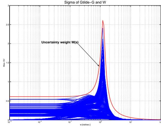
Fig. 6. Bode diagram of  $\tilde{G}(s,z) - G(s,z)$ .
